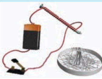
Figure 6.26 ▲ File clips fall off (do not attract) when electrical supply is disconnected
