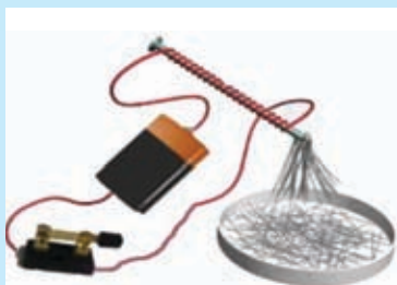
Figure 6.25 ▲ File clips are attracted when electricity is supplied
