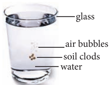
Figure 15.6 ▲ Releasing of water bubbles when a soil clod is put into water
