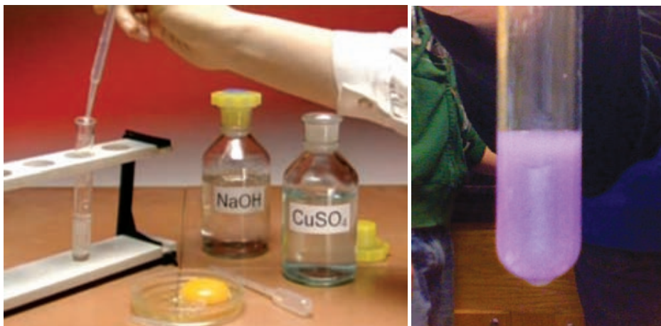
Figure 17.9 ▲ Biurette test and its observations
