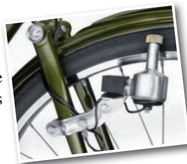
Fig:- 3.14 ▲ How a dynamo is fixed to a bicycle
