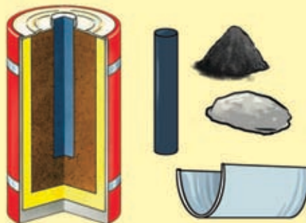
Figure :- 3.2 ▲ Contents of the dry cell
